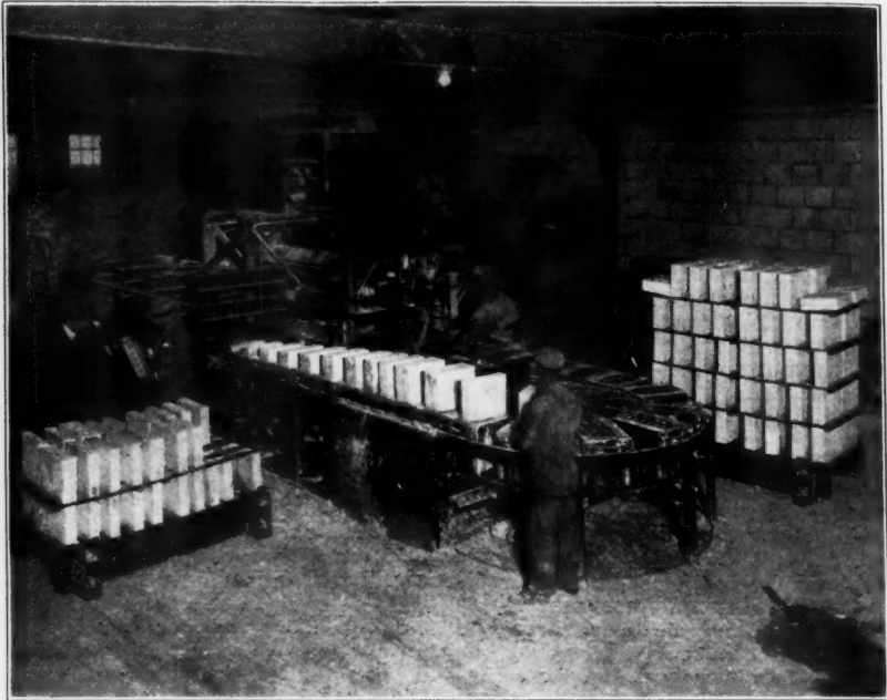
Machine Turning Out 4x6 Gypsum Tile
